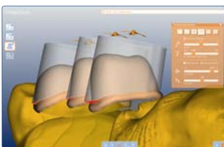
Telescope and conical primary crowns, designed in 2½ minutes per attachment
