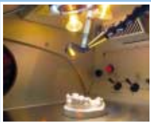
Working room with the inner operating elements: Diode ring light, Argon- and air nozzle and much more.
