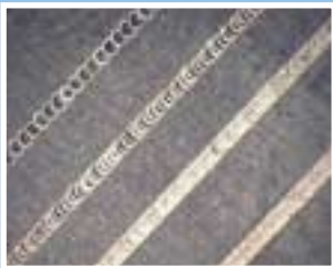
Economically lasered homogeneous and perfect welding seams thanks to pulse customization at 5, 10, 15 and 20 Hz with a constant feed.
