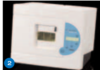
2 Place model in the Eclipse® junior VLC Curing Unit. Make sure the top of the model is below the maximum height line (row of holes in the back wall of the chamber). If this is not the case, remove stone from bottom of the model until the entire model is below this line.
